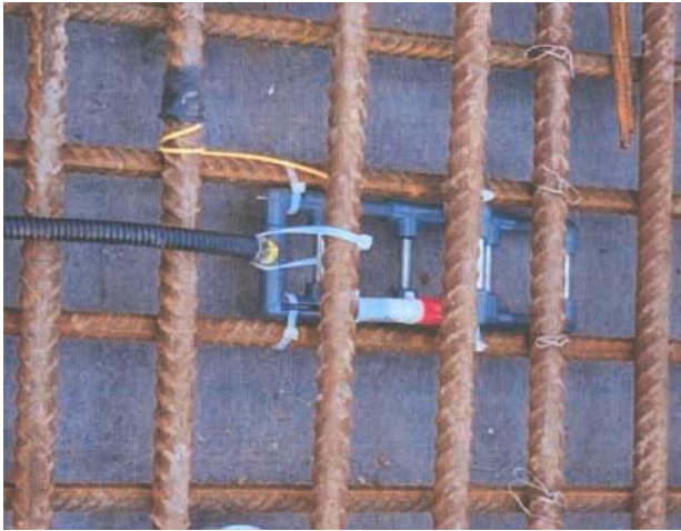
Fig.8: Corrosion sensors for monitoring of corrosion.
