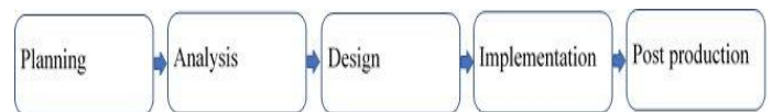
Fig. 1. SDLC for systems with stable requirements. If business requirements changes dramatically new project should be kicked off.
