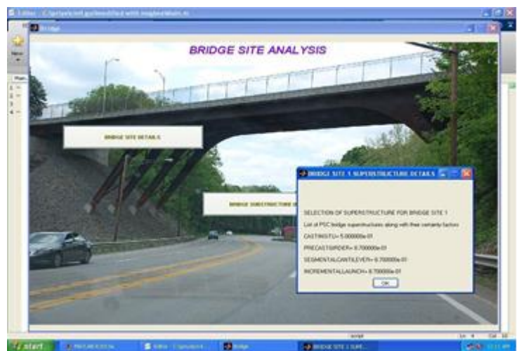
Fig. 12: Sample output of an expert system showing the suitable bridge superstructures with their certainty factors.
