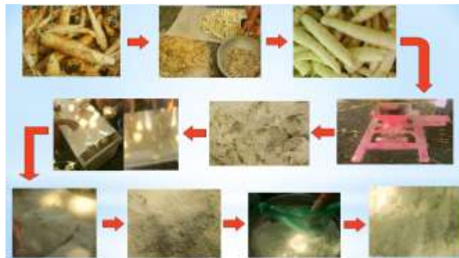
Figure 3. Process flow chart of arrowroot starch backyard processing
