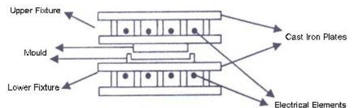
Fig. 1: The parts of mould attached to the press machine
