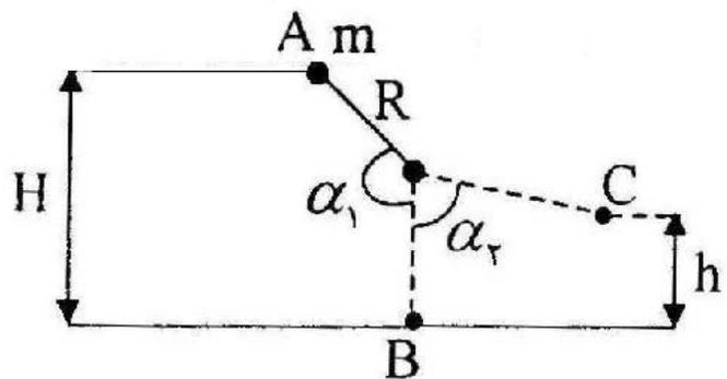
Fig. 2- The schematic pendulum used to measure the hardness of panels
