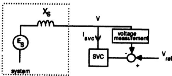
Fig. 3. Modeling of static var compensator
