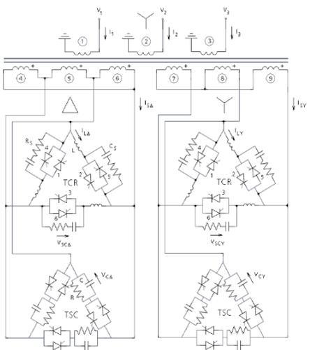
Fig. 4. Equivalent circuit of static var compensator
