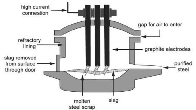
Fig. 1. Modeling of electric arc furnace
