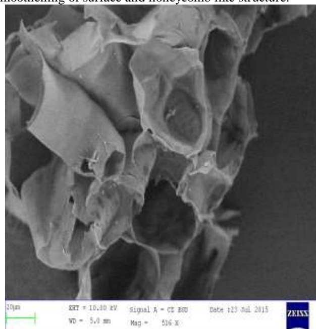
Fig.1. SEM image of original coir dust at 20µm
