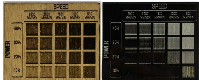
Fig. 20 Laser Engraving Calibration (15W)
