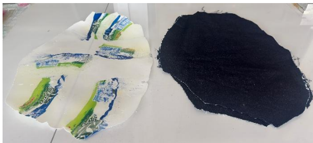
Fig. 2. PP plates and fabrics used for composite laminates.
